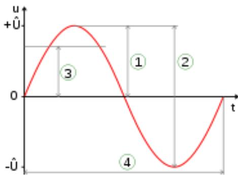
Description : A sinoidal voltage. 1 = Amplitude (peak), 2 = Peak-to-peak, 3 = RMS, 4 = Wave period
